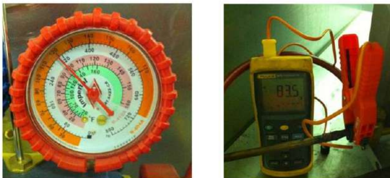
Figure 8 – Gauge Connection/Readings Liquid Line
