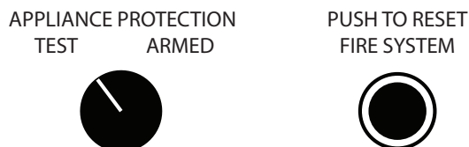
Figure 50 - Electric Control Panel “Test” Mode
